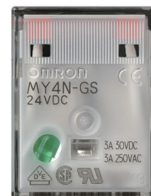
Relay with DC Coil (LED: Green)
